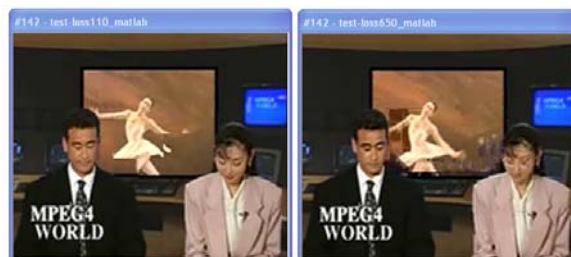
Figure 9. Impact of a lost slice for 110 bytes and 650 bytes of max. slice
