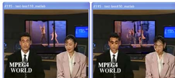
Figure 10. Impairment propagation for 110 bytes and 650 bytes of max. slice
